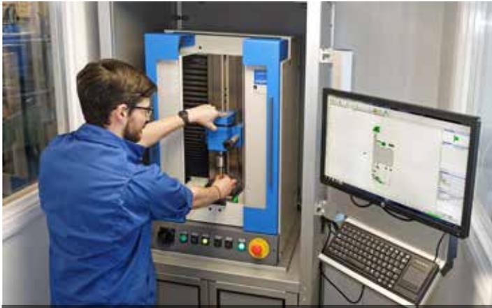
The Hommel Opticline installed in a new, dedicated inspection area at Precision Products, Rustington for automatically inspecting exterior features on rotational parts.
